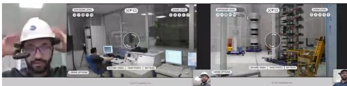
Figure 65: Remote Testing and Product Inspection with Augmented Reality - Best Transformer
